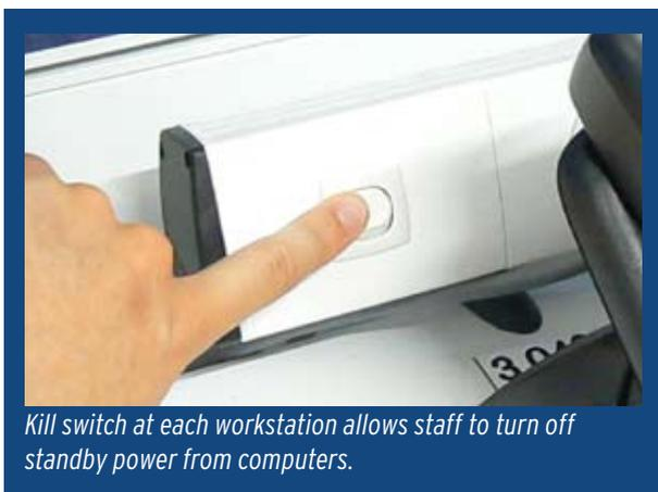
*Kill switch at each workstation allows staff to turn off standby power from computers.*
