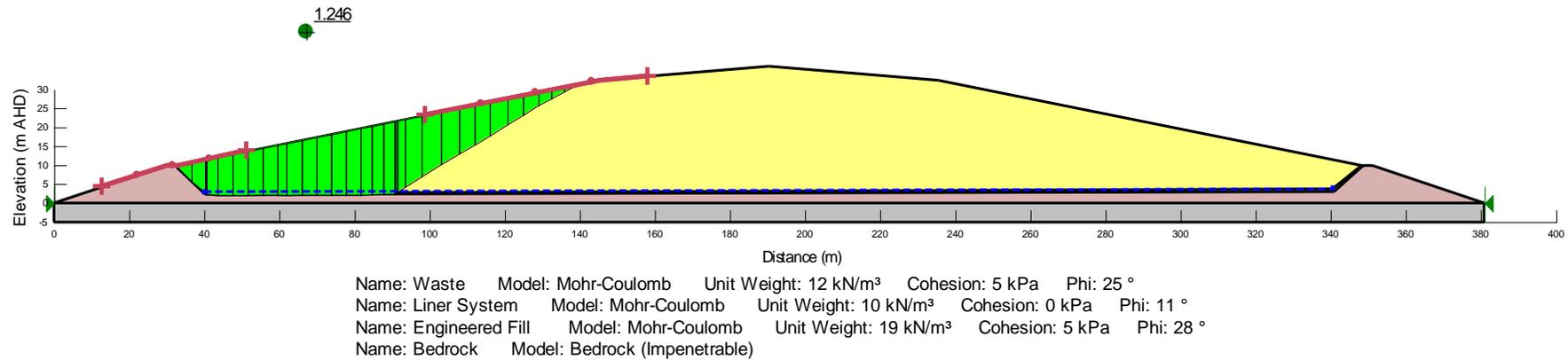
Figure 3: Case 3 – Section C Stability Analysis (seismic loading)
