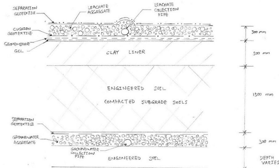
Plate 5: Proposed Groundwater Collection Layer
