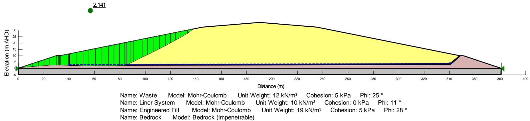
Figure 1: Case 1 - Section C Stability Analysis - Bundwall
