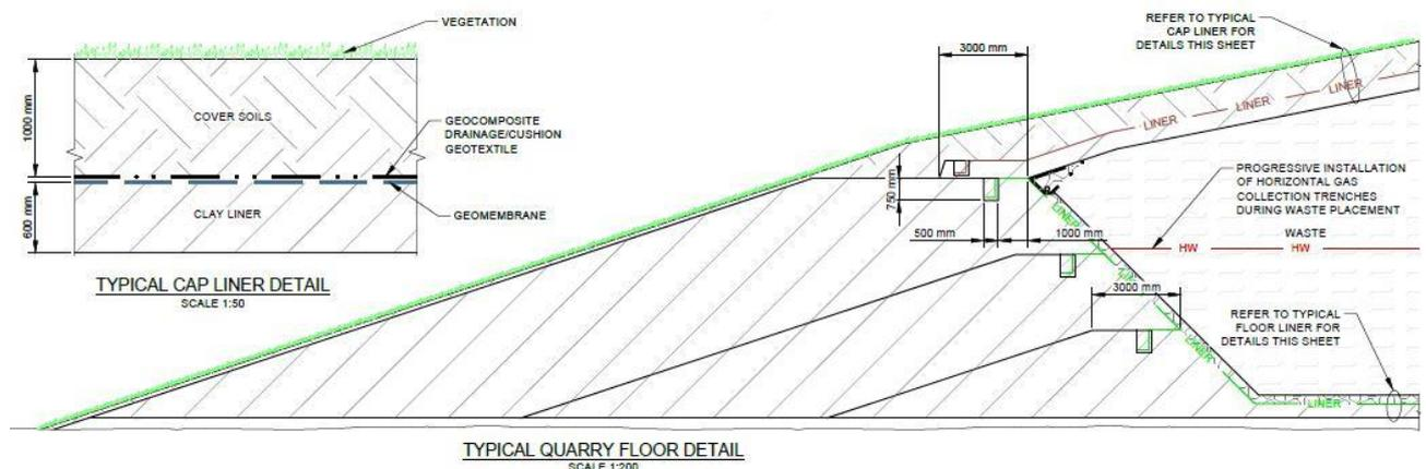
Plate 1: Typical Quarry Floor Detail, extract from Figure 27
