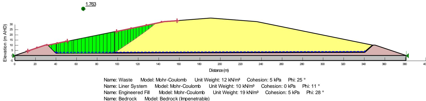
Figure 2: Case 2 - Section C Stability Analysis - Liner Interface
